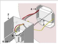
Insert ballast (5) in j-box (4) and fix bottom (2) to the j-box by means of the two screws (6).
