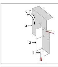
Loosen screw (1) in order to separate bottom (2) from plate (3).
