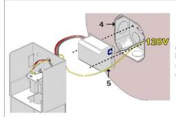
An octagonal junction box is required for this installation. The wiring must enter in j-box (4) from the side. Carry out the electrical connections: the black wire from ballast (5) must be connected to the black wire in the box and the white wire from the ballast to the white wire in the box.
