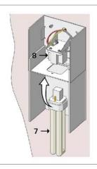
Insert bulb (7) in the proper lamp holder (8).
