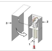
Fix plate (3) to bottom (2) by means of screw (1).
