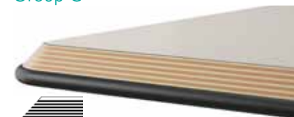
15177 1.25" 21-ply plywood edge .5" vinyl T mold bumper, black high pressure laminate top surface 3" standard radius corners
