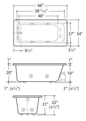
Whirlpool note: 1-horsepower motor 1 15 volt /20 amp In-line heater (optional) requires additional 1 15 -volt line
