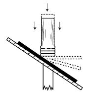
**Step 2** Fit lower side to roof pitch by raising and dropping sharply several times until fit is correct.
