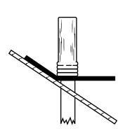
**Step 1** Install MARA-FLEX roof flashing over the vent pipe. Press down with enough force to fit the upper side to the roof pitch.
