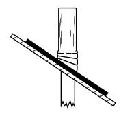
**Step 3** Ensure position is perpendicular and flange sits flush to roof.
