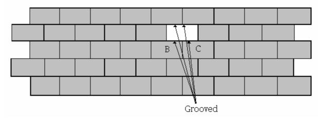
Two pieces of ¾" plumbing PVC pipe are cut 24" in length. These pieces of pipe are the replacements for the missing tongues in the system. The 24" pieces are slid in the holes formed by the removed tongue/fabricated groove openings of "B" & "C" above, as indicated by the illustration below.
