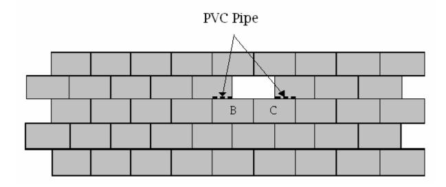
Finally, board "A" is installed into the hole with the tongue in its normal position. Using a knife blade, the PVC pipes are slid 12" laterally forming a partial tongue that will prevent the system from coming apart. This securement replacement is to be used for replacement boards in the field of the roof and is not intended as a possible replacement for normal securement as described in Technical Data Sheet 4.4.
