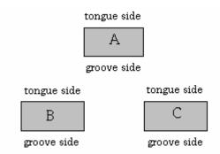
Two of the remaining boards (B & C) have their tongues removed and corresponding grooves inserted in the foam part of the LIGHTGUARD / HEAVYGUARD so that both the 4' long edges are grooved on both sides. This can easily be done with a handheld hot knife containing a long blade bent to conform to our factory groove. Boards "B" & "C" should have a cross-sectional profile as shown below.
