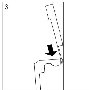
▶ Never begin by removing center SignBands when assembly incorporates multiple bands. Always begin by removing SignBands from top or bottom.
