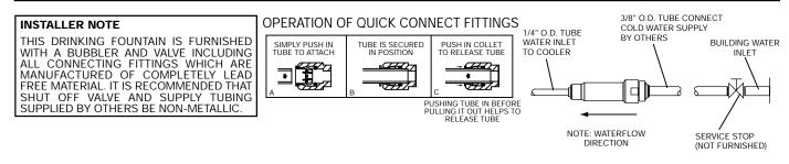
When installing EHWM214C which includes a surface mounting plate, refer to the diagrams shown below.
