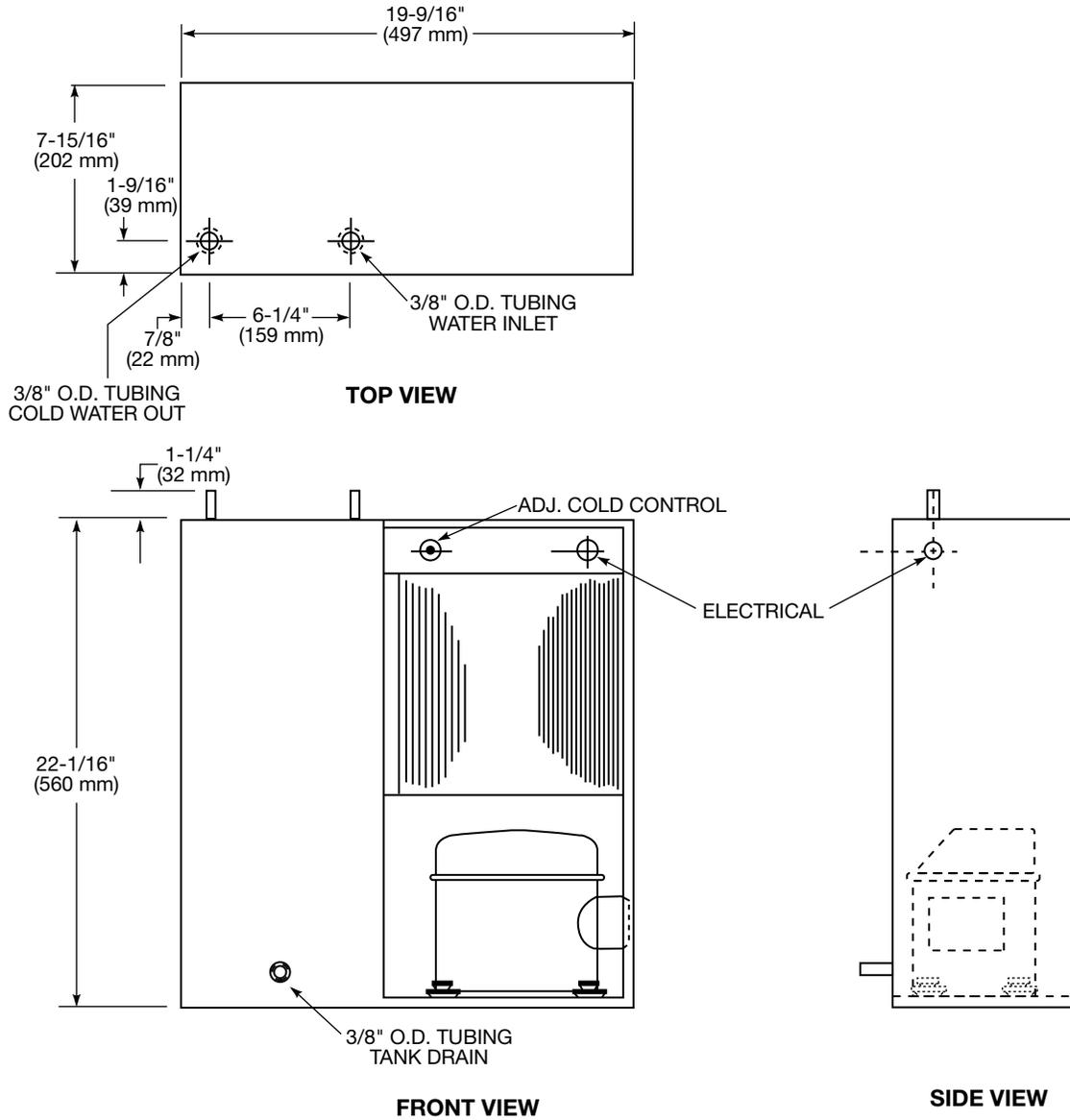
**Drain Plug:** This chiller is provided with a plastic drain plug which incorporates an o-ring seal. This fitting is designed for potable water applications and should be replaced with a suitable fitting if chiller is used with more aggressive liquids.
