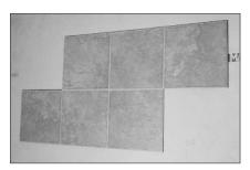
Stagger the end joints of the second row by at least one full tile pattern. Carefully align the grout lines on the panels. Pay particular attention to tile pattern repeats. Lay out panels so repetitive tile designs are not clustered
