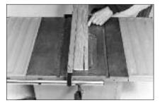
Before installation, do a calculation to determine the width of the last row of planks. If it is less than 1-1/2" wide, split the difference between the starter row and the last row. In any case, you will most likely be required to cut the last row of planks to width with a table saw equipped with a plywood cutting blade.
