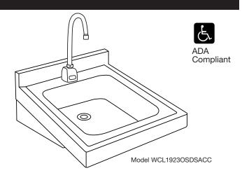
line. Control circuit is solid state, has adjustable sensor range (6" [152mm] preset to 30" [762mm]), shut off delay preset at 1 second and field adjustable to 2, 4 or 8 seconds, and automatic time-out feature (to prevent sink overflow) is preset at 0 seconds and is field adjustable to 15, 30 or 60 seconds.
