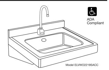
and 3/8" (10mm) stainless steel braided 12" (305mm) supply line. Control circuit is solid state, has adjustable sensor range (6" [152mm] preset to 30" [762mm]), shut off delay preset at 1 second and field adjustable to 2, 4 or 8 seconds, and automatic time-out feature (to prevent sink overflow) is preset at 0 seconds and is field adjustable to 15, 30 or 60 seconds.
