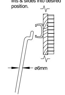
4. Installation complete. Reposition as needed. Friction holds rods in place.
