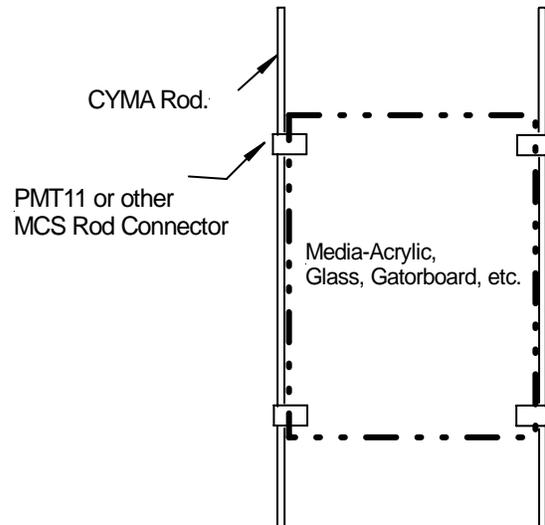
3. Pivot CYMA rod so that the "S" shaped groove lifts & slides into desired position.
