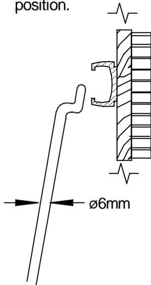
4. Installation complete. Reposition as needed. Friction holds rods in place.
