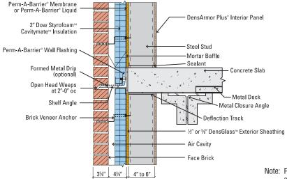
Note: Perm-A-Barrier® WB Primer is required for application of membrane to DensGlass™
