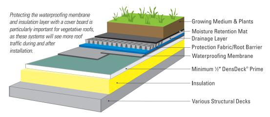
a fire barrier. In this way, the use of one cover board solves numerous roofing problems for the architect and property owner. In terms of labor costs, DensDeck® Prime provides a stronger and more economical installation by reducing the damage during installation. The product also eliminates the need for a field primer and reduces the number of fasteners required to achieve high wind uplift values.
