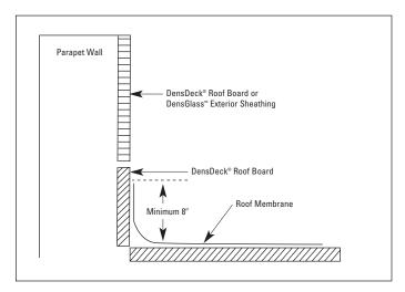
In most membrane roofing systems, membranes must extend up the inside of a parapet wall at least 8 inches, and the membrane must be backed by a suitable roofing substrate.
