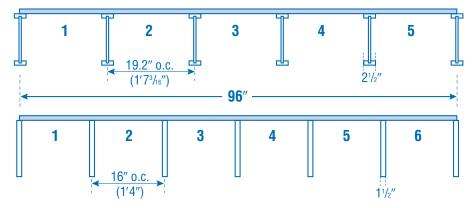
The engineered lumber floor system shown above yields almost 40% more subfloor support and fastening surface than the ordinary lumber system while reducing the amount of wood used in the floor.
