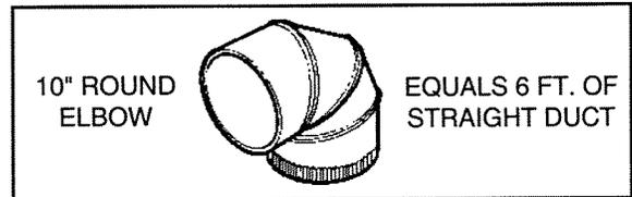
3. The system will operate most efficiently when the ductwork does not exceed 40 feet of equivalent duct. The illustration, above, shows equivalent feet of a 10" round elbow. The number of feet of straight duct plus the equivalent feet of elbows to be used should equal 40 feet or less.
