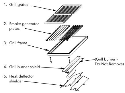
Clean greasy parts with a household grease solvent such as household ammonia and water. If necessary, a soap filled steel wool pad can be used on the grill frame shield, grill burner, and grill heat deflector.
