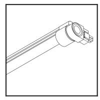
**Bee**Rail <sup>™</sup> - 1.125" Ø extruded aluminum micro-spine designed for exposed bulb or diffuser attachment to structure. Hub design features 370° rotation, angle-gauge and lock-screw. Brushed and clearcoated aluminum finish. Mounts to Single or Double Arm.
