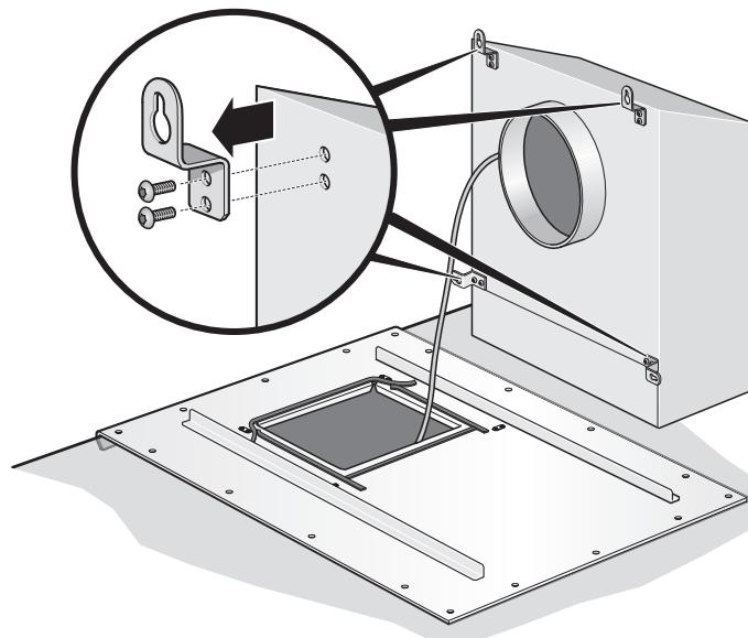
Mounting the blower on the roofplate
