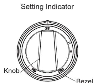
**Figure 3: Standard Burner Control Knob**
