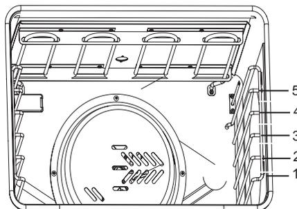
Figure 1: Oven Rack Positions
