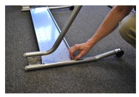
Step 2: Once both legs are attached to the modesty panel, attach the flip beam to the legs. Secure all bolts that hold flip beam and modesty panel.
