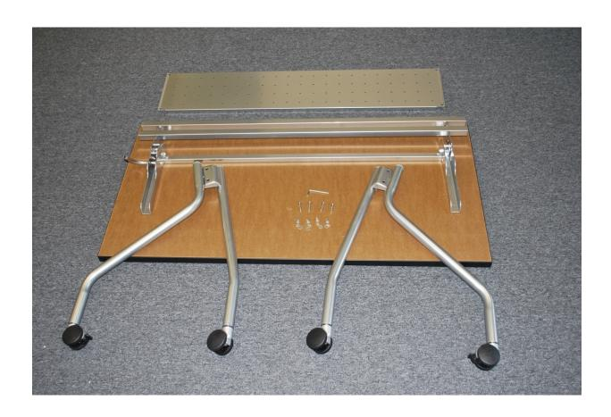
Step 1: Set the modesty panel on the floor with the troth on the bottom. Attach modesty panel to the legs by setting the legs on the floor and aligning modesty panel holes with the holes on the legs. Use short screws for attachment, but do not tighten the screws until the flip beam is in place.
