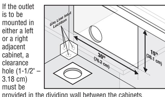
**NOTE:** The free length of the appliance's power cord is approximately 46" (116.8 cm). In planning the location of the clearance hole and outlet, the cord's length should be considered.
