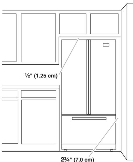
To ensure proper ventilation for your refrigerator, allow for a 1/2" (1.25 cm) space at the top and behind the refrigerator. If your refrigerator has an ice maker, allow extra space at the back for the water line connections. When installing your refrigerator next to a fixed wall, leave 2-3/4" (7.0 cm) minimum space between the refrigerator and wall to allow the door to swing open.
