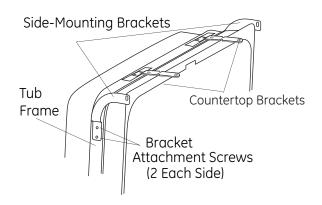
• If you are installing the dishwasher under a counter with a short overhang, the countertop brackets may extend beyond the edge of the counter. If this is the case, remove the excess length by repeatedly bending the brackets at the notches until they break off.
