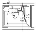
Waste Tee Installation Figure Z
