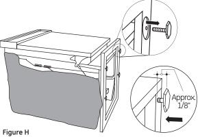
• Screw leveling legs back into the dishwasher frame, approximately 1/8" from frame as shown.
