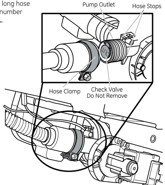
**Tip: Avoid unnecessary service charges. Make a leak free connection**
