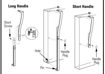
After removing the handle: Move the small plug buttons from the top right side of the door top and insert them into the holes on the opposite side.
