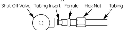
**NOTE:** Overtightening will cause the tubing to separate from the fitting.
