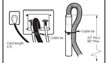
**NOTE:** Drain hose MUST be secured to drain facility in all cases.
