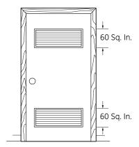
When louvers or registers are placed in door openings, the free air openings of the louvers or registers must equal 120 square inches.
