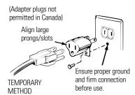
**CAUTION**: Attaching the adapter ground terminal to the wall receptacle cover screw does not ground the appliance unless the cover screw is metal, and not insulated, and the wall receptacle is grounded through the house wiring.
