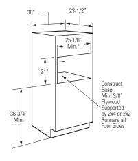
all models. The amount of overlap on the sides depends on the actual cutout width. Allow 1-1/4" case trim overlap on the top for models PSB2200 and PSB2201 and for models ZSC2200, ZSC2201 and ZSC2202.
