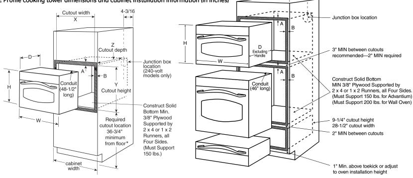
A=Allow 7/8" overlap of oven over bottom and 1/4" overlap at top edges of cutout.
