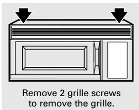
To remove the charcoal filter, disconnect power at the main fuse or circuit breaker panel or pull the plug.
