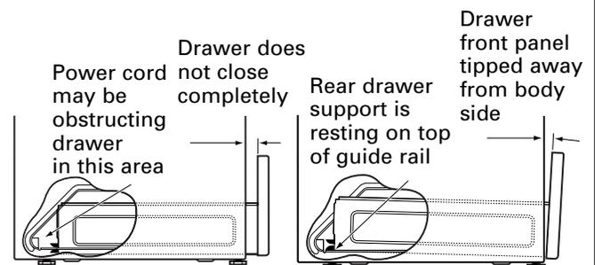
Remove and replace, making sure the power cord is not obstructing the drawer and/or the rail is in the guide.
