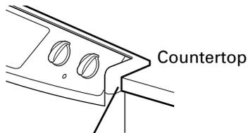
Make sure the edge of the countertop fits flush against the end of the front control panel
