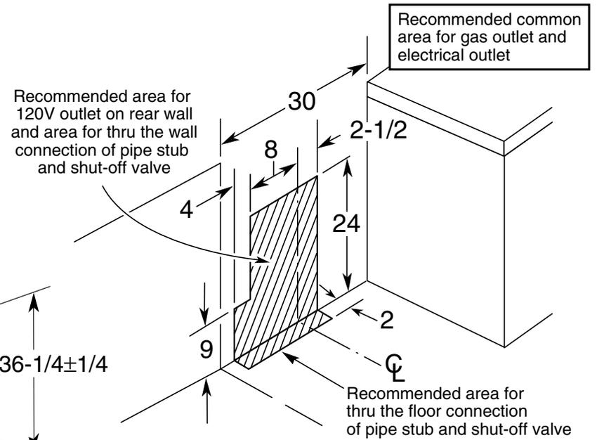
\*Dimension from the wall to the front of the closed door handle is 28-1/4". Depth to the front edge of cooktop 25-1/4".
