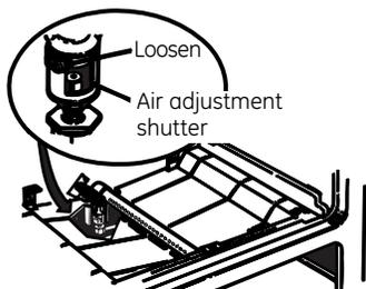
The shutter for the bottom (oven) burner is near the back wall behind the drawer. Remove the drawer. See the *Care and cleaning of the range* section.
