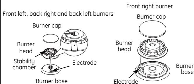
Make sure the slot in the burner head is positioned over the electrode.
