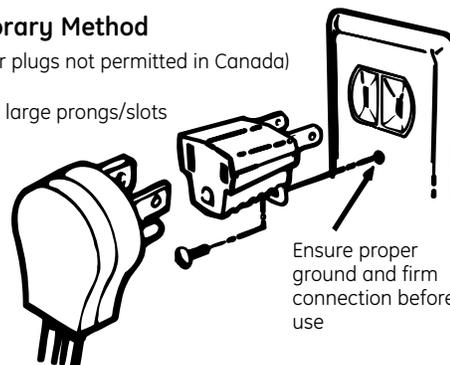
**CAUTION:** Attaching the adapter ground terminal to the wall receptacle cover screw does not ground the appliance unless the cover screw is metal, and not insulated, and the wall receptacle is grounded through the house wiring. The customer should have the circuit checked by a qualified electrician to make sure the receptacle is properly grounded.
