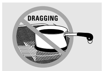
Do not slide cookware across the cooktop because it can scratch the glass. The glass is scratch-resistant, not scratchproof.
