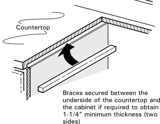
The Standard Installation of this Drop-In Range is to hang by the countertop on the side metal flanges under cooktop. **This Range must not be installed on a base or sub structure (2"x 4" support).**
