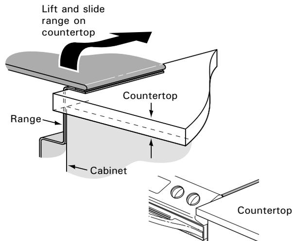
Make sure the edge of the countertop fits flush against the end of the Front Control Panel
