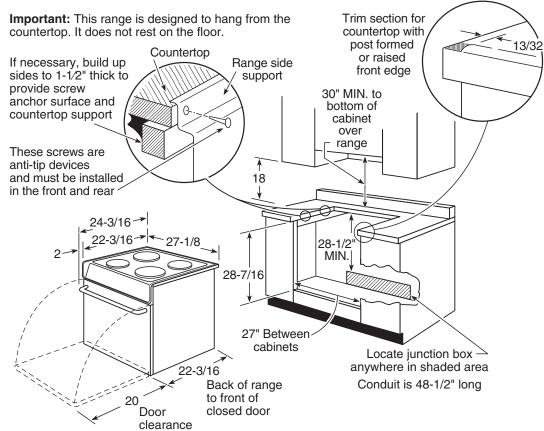
**Note:** Cabinets installed adjacent to drop-in electric ranges must have an adhesion spec of at least a 194°F temperature rating.
