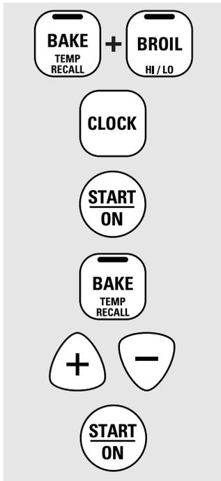
When the display shows  $\supset$  the oven is set in Sabbath. When the display shows  $\supset C$  the oven is baking/roasting.
