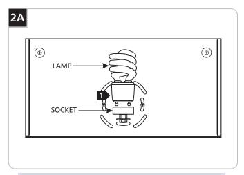
**CAUTION:** To reduce the risk of a burn or electric shock during relamping, disconnect the power to the fixture by turning the wall switch off.
