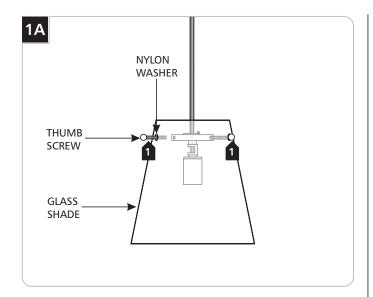
1 Line up the glass shade holes with the disk holes and secure the glass shade to the disk with provided thumb screws and nylon washers.
