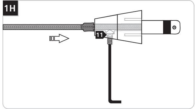
**11** Firmly tighten the set screw on the conical connector.
