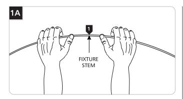
1 Simply bend the fixture stem to the desired shape by hands.
