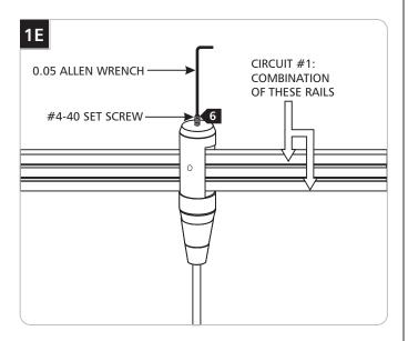
6 Select circuit #1 by fastening the #4-40 set screw on top of the housing very tight with the 0.05 Allen wrench.
