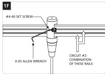
When using circuit #2, remove the #4-40 set screw from top of the housing and screw it into the side with the 0.05 Allen wrench very tight.
