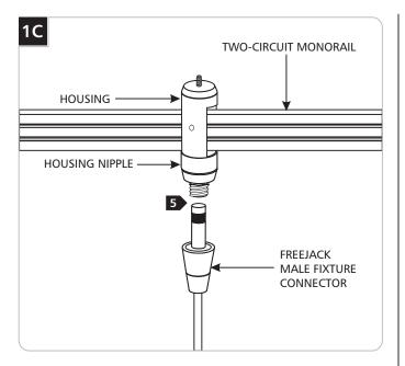
Screw the FreeJack male fixture connector onto the housing nipple.
