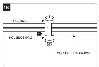
4 Screw the housing nipple to the housing tight. Make sure not to cross thread the housing nipple to the housing.
