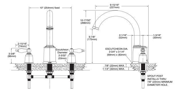
NOTE: THE INSTALLATION SHOWN IS FOR TILE DECKS, THIS VALVE WILL ALSO FIT STEEL, CAST IRON OR PLASTIC DECKS
