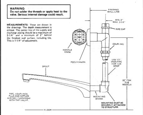
CAUTION: Always turn water OFF before disassembling the valve. Open both valve handles to alleviate water pressure to insure that COMPLETE water shut-off has been accomplished.
