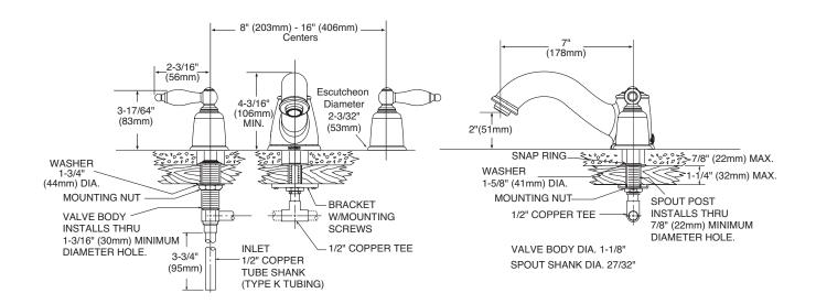
NOTE: THE INSTALLATION SHOWN IS FOR TILE DECKS, THIS VALVE WILL ALSO FIT STEEL, CAST IRON OR PLASTIC DECKS
