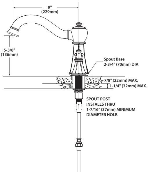
**NOTE:** THE INSTALLATION SHOWN IS FOR TILE DECKS, THIS VALVE WILL ALSO FIT STEEL, CAST IRON OR PLASTIC DECKS
